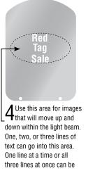
projected here using the fixture shutters. Maximum available image area: 1 1/2" (L) x 3" (W) 38.1mm (L) x 76.2mm (W) **5** Use this area for images that will disappear at the top of the light beam. Use in conjunction with area #6 to have one pattern completely replace another pattern in the center of the light beam. Maximum available image area: 5/8" diameter
