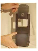
Continue sliding the gobo into the Smart Move<sup>®</sup> Vertical until the holes in the gobo line up with the screw holes on the gobo carrier plate. Screw two Phillips head screws until tight. Do not Over tighten!
